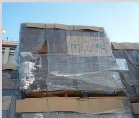
Conventional stretch wrapping method - Water runs down the straps and damages the product.
