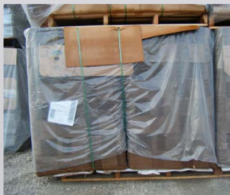
Conventional wrapping with loose bags - Lower part of bale exposed to outdoor elements.
